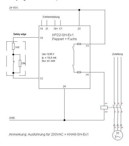
Example (symbolic representation) of the interconnection with a safety relay: terminals S10 and S12 are intended for IS-equipment; as an alternative, the safety edge can also be supplied with the resistor circuit.
