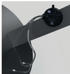
Keep antenna clear off the metallic surface
